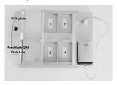
Figure 24. Placement of PCR plate (or strips) and PyroMark Q96 Plate Low or PyroMark Q96 HS Plate on the PyroMark Q96 Vacuum Workstation. The marked positions contain 70% ethanol (1), PyroMark Denaturation Solution (2), PyroMark Wash Buffer (3), and high-purity water (4).
