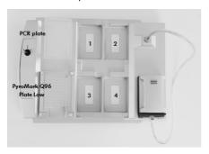
Figure 13. Placement of PCR plate (or strips) and PyroMark Q96 Plate Low on the PyroMark Q96 Vacuum Workstation. The marked positions contain 70% ethanol (1), PyroMark Denaturation Solution (2), PyroMark Wash Buffer (3), and high-purity water (4).
