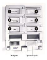
Figure 23. Positions on the PyroMark Q24 Vacuum Workstation.
