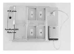
Figure 18. Placement of PCR plate (or strips) and PyroMark Q96 HS Plate on the PyroMark Q96 Vacuum Workstation. The marked positions contain 70% ethanol (1), PyroMark Denaturation Solution (2), PyroMark Wash Buffer (3), and high-purity water (4).
