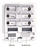
Figure 9. Placement of PCR plate (or strips) and PyroMark Q24 Plate on the PyroMark Q24 Vacuum Workstation. The marked positions contain 70% ethanol (1), PyroMark Denaturation Solution (2), PyroMark Wash Buffer (3), and high-purity water (4, 5). P: Parking position.
