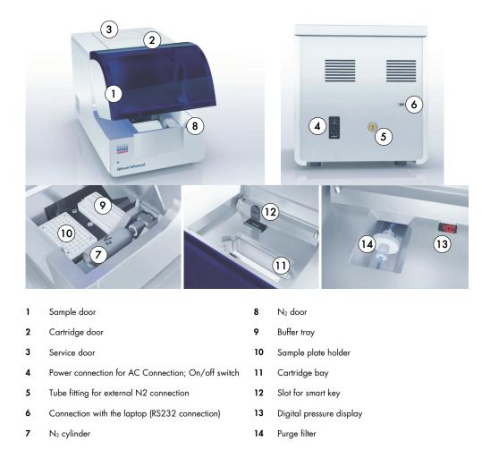
**Note**: If using an external  $N_2$  source, the output pressure must not exceed 75 psi. The QIAxcel Advanced instrument is equipped with an internal regulator that regulates the pressure generated by the external  $N_2$  source to approximately 35 psi (30–40 psi), which is the instrument's operating pressure.
