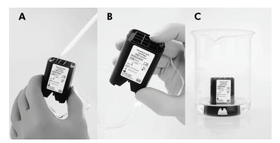
Cleaning the PyroMark Q96 Cartridge. A Filling the compartments with high-purity water. B Placing pressure on compartments.
