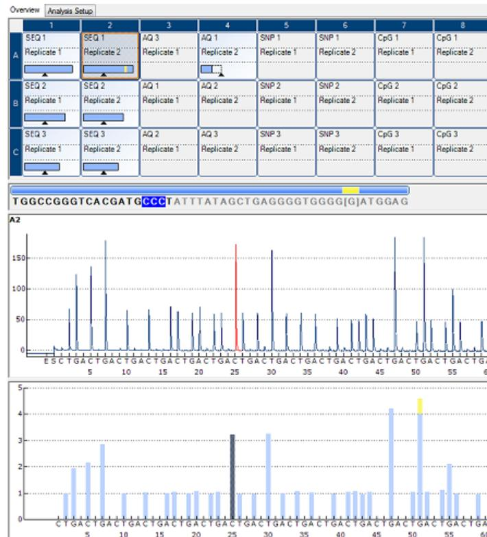
When a base is selected in the base-called sequence, the corresponding peak is highlighted in both Pyrogram areas, and vice versa.
