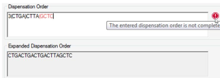
The error “The entered dispensation order is not complete” is caused by a missing or incorrect positioned parenthesis. In this example, a closing parenthesis is missing.
