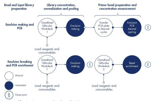
Figure 1. Workflow: bead preparation and enrichment for NGS.
