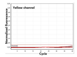
**Figure 3. The PCR is inhibited.** No amplification of the three samples in the green channel (left) or the internal control in the yellow channel (right). All curves lie along the baseline and do not exceed a preset threshold.
