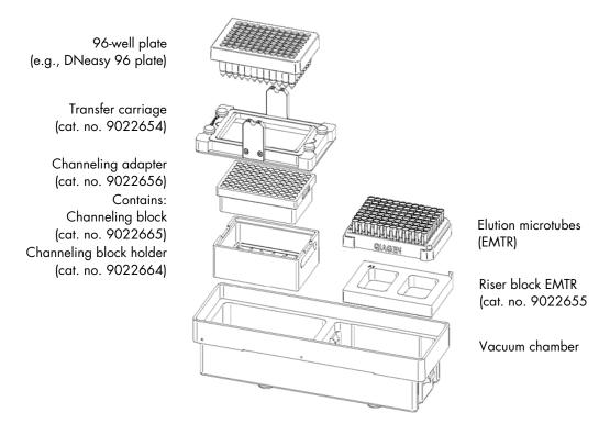
Figure 1. Assembling the vacuum chamber.
