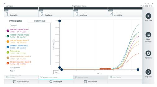
Figure 17.Amplification Curves screen (PATHOGENS tab).
