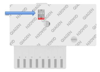
Figure 3. Sample inspection window (blue arrow).
