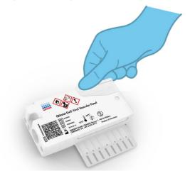
Figure 9. Closing the sample lid of the main port.
