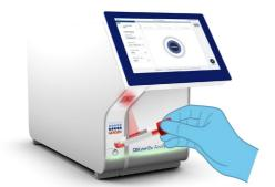
Figure 11.Scanning sample ID bar code.
