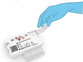
Figure 6.Opening the sample lid of main port.
