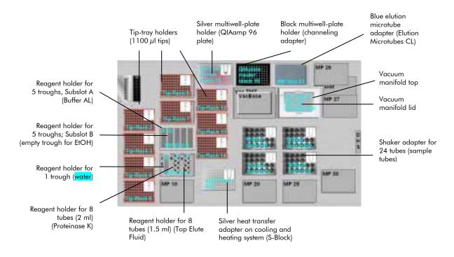
Figure 2. Worktable overview. A schematic diagram of worktable setup.
