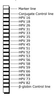
Figure 1. Schematic of the genotyping strip. A marker line (Marker line) is drawn at the top of the strip for orientation. Two control lines (Conjugate Control line,  $\beta$ -globin Control line) are included.
