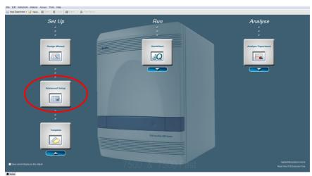
Figure 25. Starting a new experiment using Advanced Setup.
