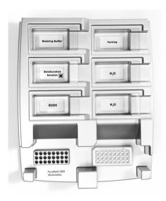
Figure 2. Placement of PCR plate (or strips) and PyroMark Q24 plate on the vacuum workstation.
