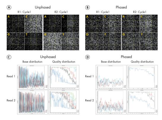
Figure 3. QIAseq 165/ITS Panels employ phased primers to increases base diversity and quality scores. Fluorescent images (top row) taken from the first cycle of read 1 (R1) showing uneven base distribution in an unphased primer run A and more even base distribution in a phased primer run B. Low base diversity and read quality scores (bottom row) are apparent in a run using unphased V3V4 primers C and significantly improved using phased V3V4 primers D.
