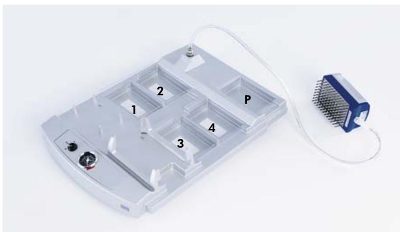
**Figure 3. PyroMark Q96 Vacuum Workstation.**
