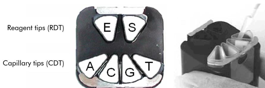
**Arrangement of tips in the PyroMark Q96 Capillary Tip Holder.**
