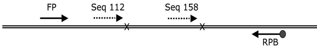
**Figure 1. PyroMark APOE assay.** PCR primers are shown as solid arrows, while sequencing primers are shown as dashed arrows. **FP:** Forward primer; **RPB:** Reverse biotinylated primer; **Seq:** Sequencing primer.
