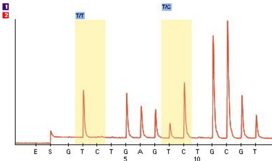
Pyrogram trace obtained after analysis of samples with T/T genotype in SNP 112 and T/C genotype in SNP 158.
