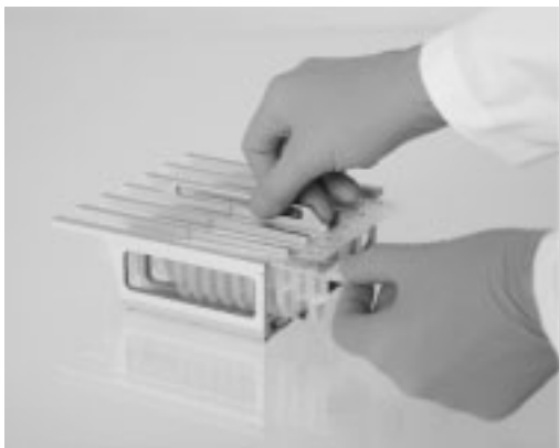
Figure 3. Ease of worktable setup using reagent cartridges. A A sealed, prefilled reagent cartridge. Fill levels vary, depending on the type of reagent cartridge. B Loading reagent cartridges into the cartridge rack. The cartridge rack itself is labeled with an arrow to indicate the direction in which reagent cartridges must be loaded.
