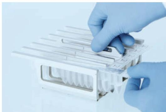
**Figure 9. Loading the reagent cartridge rack.** The cartridge rack itself is labeled with an arrow to indicate the direction in which reagent cartridges (RCB) must be loaded.
