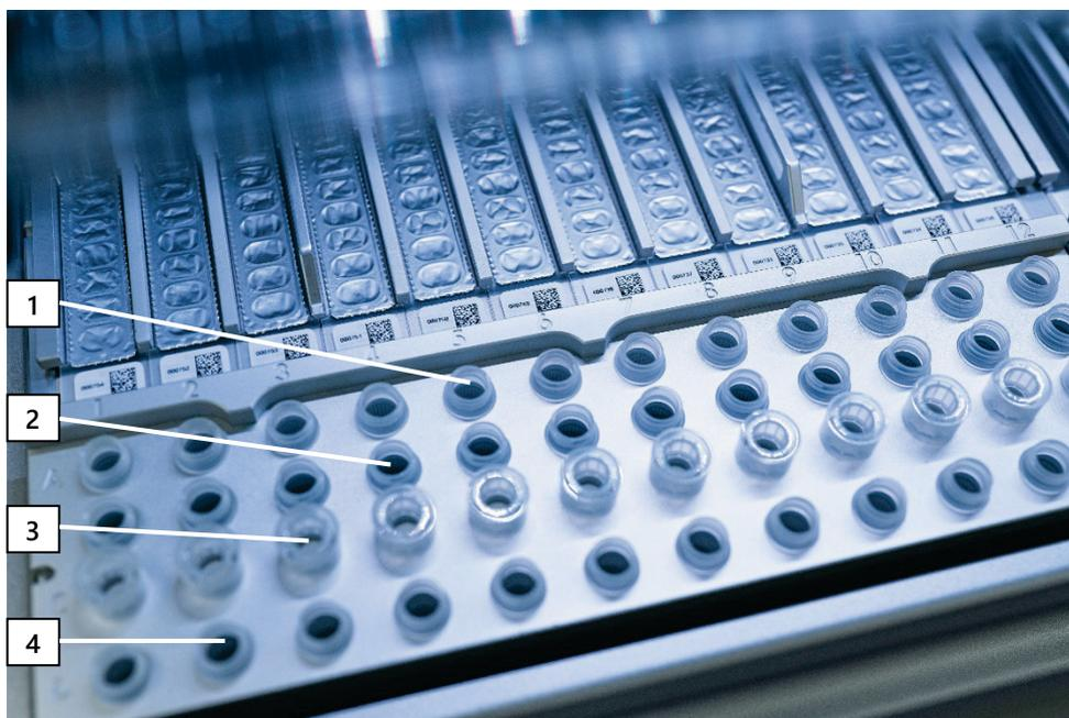
**Figure 5. Worktable of an EZ2 Connect MDx instrument.** (1) Sample tubes (ST) (2 ml) loaded into row A. (2) Empty or optional: Tube (2 ml) containing 80% Ethanol for optional wash step, loaded into row B. (3) Disposable tip holders (DTH) containing disposable filter-tips (DFT) loaded into row C. (4) Elution tubes (ET) (1.5 ml) loaded into row D.
