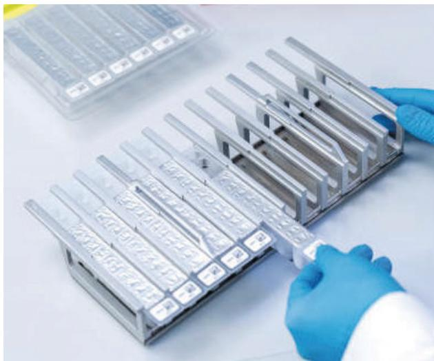
**Figure 3. Reagent cartridge rack.** The cartridge rack itself is labeled with an arrow to indicate the direction in which reagent cartridges (RCB) must be loaded.
