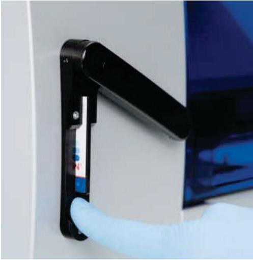
**Figure 7. EZ1 Card completely inserted into EZ1 Card slot.**
