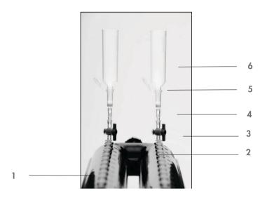
Figure 2. Setting up the QIAvac 24 Plus with QIAamp Mini columns using VacValves, VacConnectors, and Column Extenders.
