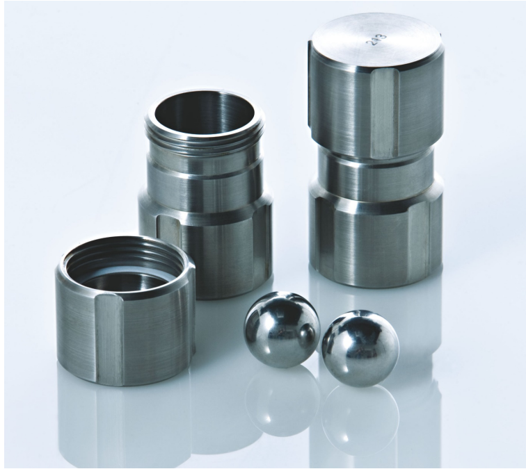
Figure 12. Grinding Jar Set, Stainless Steel. Each 10 mL jar is made of stainless steel and contains a 20 mm diameter stainless steel grinding ball.
