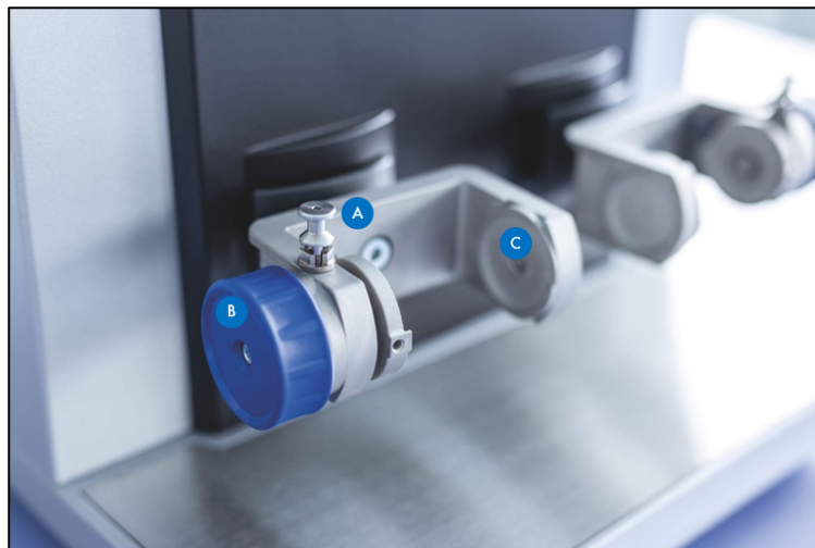
Figure 20. Left-hand clamp of the TissueLyser III. A Locking pin. B Handwheel. C Indentation in clamp.
