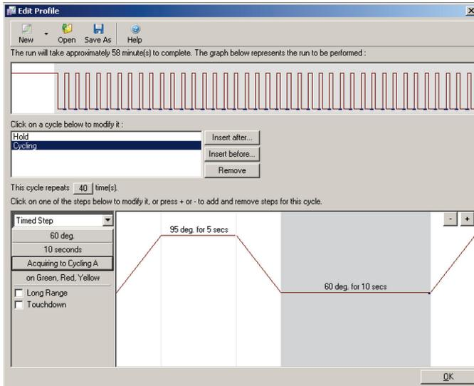
**Two-step cycling. PCR requires 40 cycles. Each cycle consists of 2 steps: 95°C for 5 s (denaturation step) and 60°C for 10 s (annealing/extension step).**
