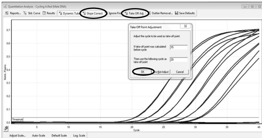
Slope correction and Take Off Point Adjustment tool.
