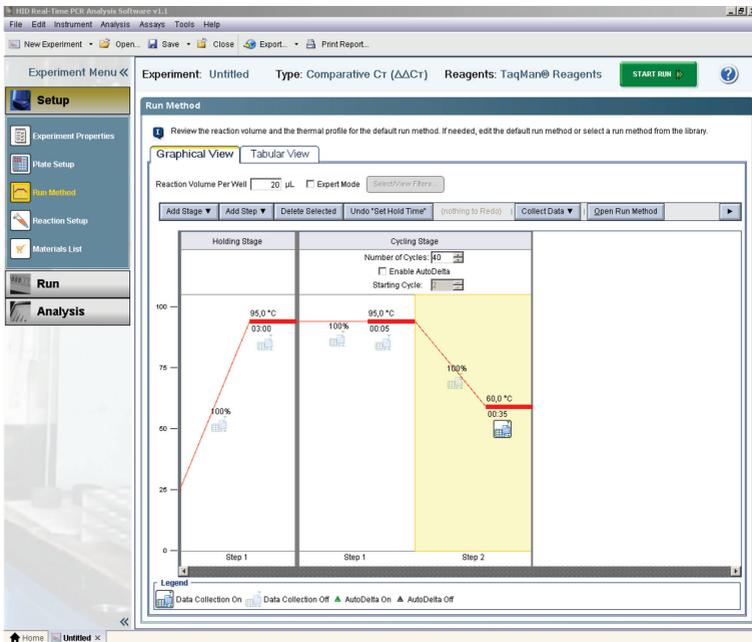
**Adjusting the thermal profile (HID Real-Time PCR Analysis Software v1.1).**
