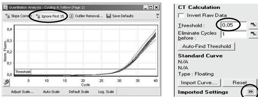
Setting the  $C_T$  value for the Yellow Channel using the Import tool.
