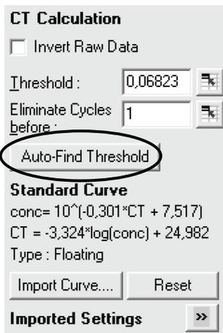
Setting the  $C_T$  value for the Green Channel using the Auto-Find Threshold.
