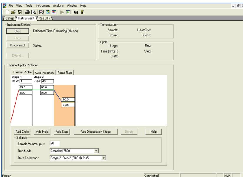
**Adjusting the thermal profile (SDS Software Version 1.4).**
