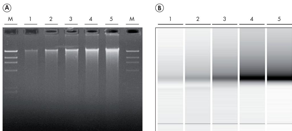
**Figure 1. Electrophoresis of samples from a dilution series. A** Lanes 1–5: gDNA samples at respective concentrations of 10, 25, 50, 75, and 100 ng/ $\mu$ l run on a 1% agarose gel for 150 min at 80 V. **Lane M:** lambda HindIII size marker. **B** The same samples run using a QIAxcel DNA Screening Cartridge and the AM900 method.
