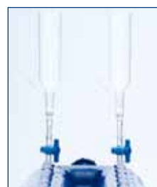
QIAamp Mini columns. shown with tube extenders for processing up to 5 ml blood sample on the QIAvac 24 Plus.
