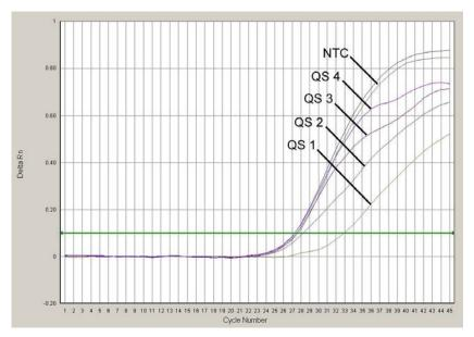
Fig. 24: Detection of the Internal Control (IC) by measurement of the VIC fluorescence signal (ABI PRISM 7000 SDS) with simultaneous amplification of the Quantitation Standards (EBV LC/RG/TM QS 1 - 4). NTC: non-template control (negative control).
