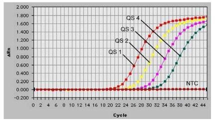
Fig. 25: Detection of the Quantitation Standards (EBV LC/RG/TM QS 1 - 4) by measurement of the FAM fluorescence signal (ABI PRISM 7700 SDS). NTC: non-template control (negative control).
