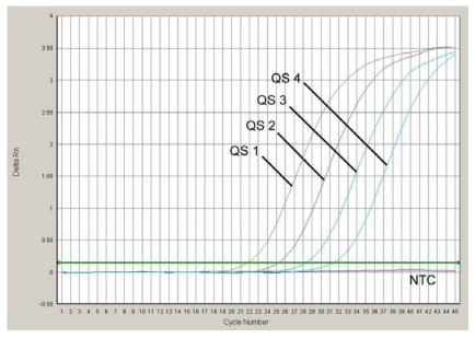
Fig. 23: Detection of the Quantitation Standards (EBV LC/RG/TM QS 1 - 4) by measurement of the FAM fluorescence signal (ABI PRISM 7000 SDS). NTC: non-template control (negative control).
