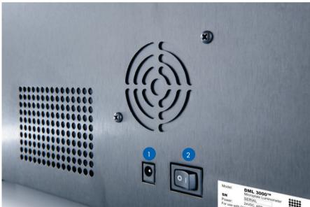
Figure 13. View of the power connection and the power switch. (1): Power connection port (2): Power switch
