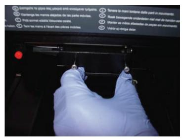
Figure 40. Removing the optical mask.
