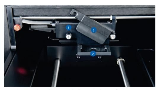
Figure 7. Close-up view of the optical head. (1): Optical head (2): Optical mask (3): Optical mask retainer
