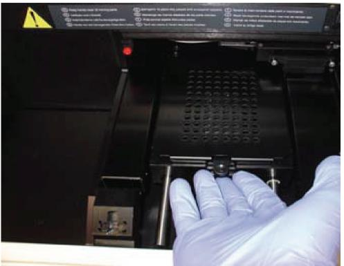
Figure 36. Pushing the plate carrier
