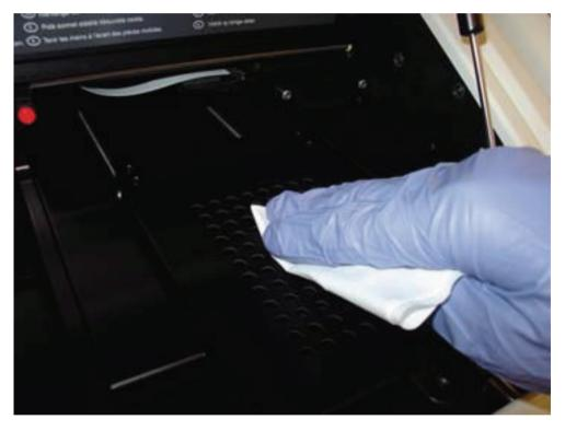
Figure 33. Wiping the top of the plate mask
