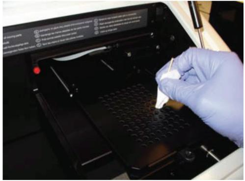
Figure 35. Cleaning the plate mask openings
