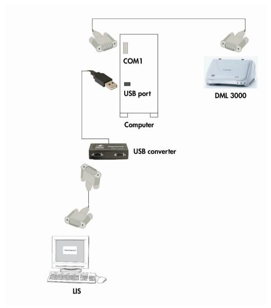
Figure 25. Diagram of connecting a DML 3000 with a LIS.
