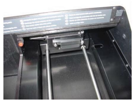
Figure 38. The optical head in the centered position
