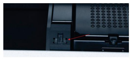
Figure 6. Close-up view of the optical sensor
