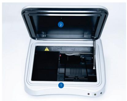
Figure 5. View of the optical sensor when the access door is opened. (1): Optical sensor (2): Flag
