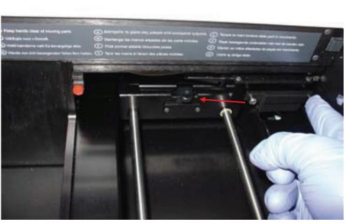
Figure 37. The optical head in the home position
