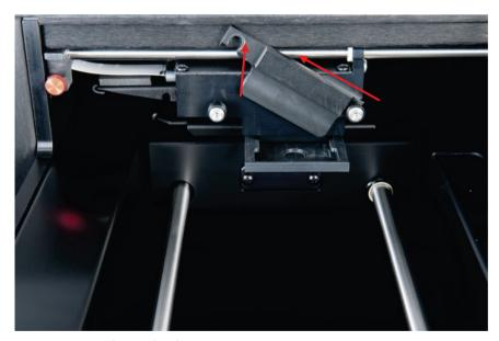
Figure 39. Removing the optical mask retainer
