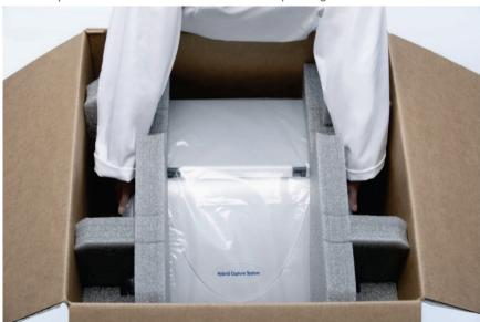
Figure 17. Removing the DML 3000 from the shipping box
