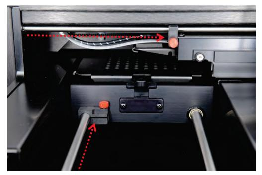
Figure 29. View of the transport locks in the secured position.
