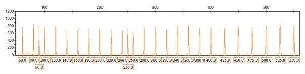
Figure 5. Electropherogram of the DNA Size Standard 550 (BTO), fragments with lengths in bp
