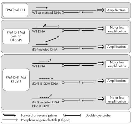
Figure 1. Results obtained with the primers and probe mixes in the *therascreen* IDH1/2 RGQ PCR Kit. The same principle shown to detect *IDH1* R132H applies for *IDH1* R132C and *IDH2* R172K.
