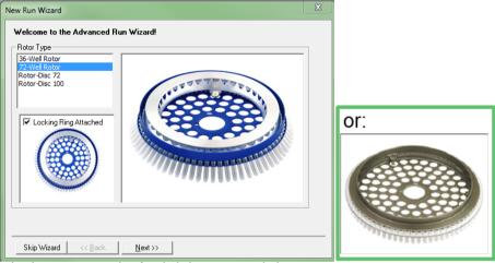
Select the correct Rotor and confirm the locking ring is attached.
