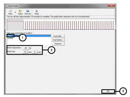
Figure 5. Initial activation of the hot-start enzyme.
