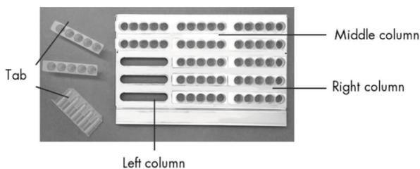
**Figure 1. Correct loading of 5-tube strips in the tube strip tray.**
