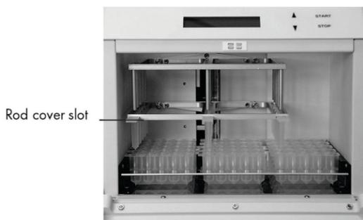
**Figure 2.** Rod cover slot.
