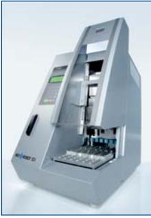
**Figure 1. The BioRobot EZ1 workstation processes up to 6 haplotype-specific extractions.**
