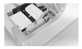
Preparing the buffer tray and inserting the buffer tray into the buffer tray holder.
