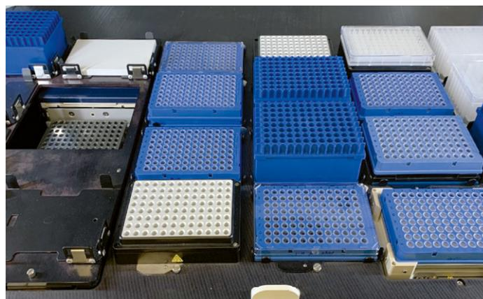
**Figure 2. Example of the deck layout for the QIAseq DIRECT Enhanced protocol setup during cDNA synthesis – the first step of the workflow on the Sciclone G3 NGSx iQ workstation.**
