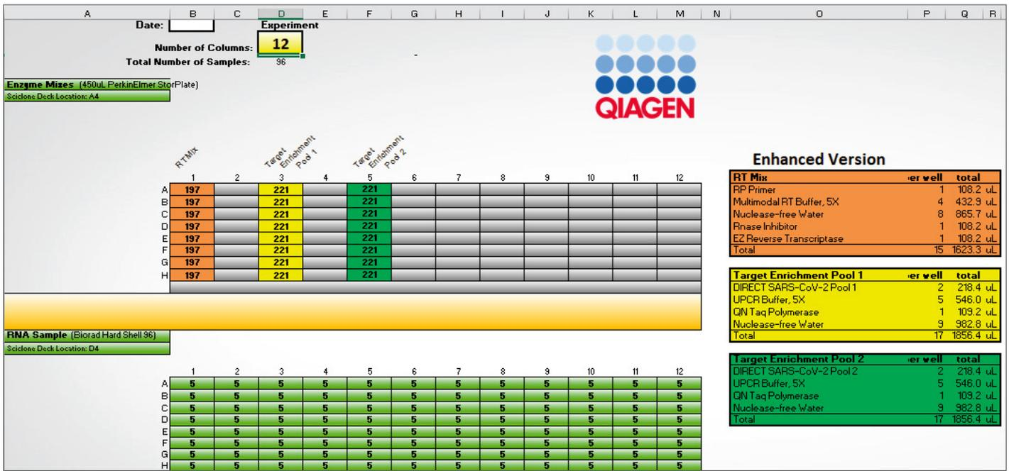
**Figure 3. An example of the Excel® workbook describing the recipes and volumes required for the different master mixes.** The number of columns can be adjusted to support a variety of sample quantities throughout the automated workflow.
