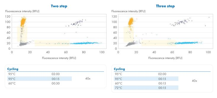
Figure 8. Transition from two- to three-step thermal cycling can improve separation. 100 copies/µl wild-type gDNA samples were tested with CDH1 (FAM)/TERT (HEX) in a duplex reaction. QIAcuity Probe PCR Master Mix was used. The cycling parameters are as indicated in the table, and the standard QIAcuity imaging setup was used. This adaptation improves the cluster separation.
