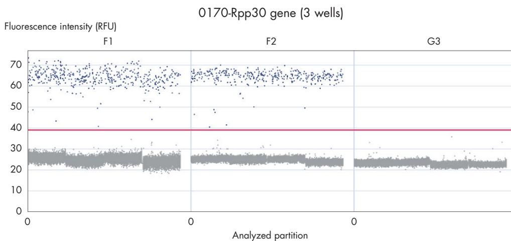
Figure 2. Fluorescence intensities as measured by the QIAcuity instrument. 0170-Rpp30 gene: F1 = Positive donor; F2 = Negative donor; G3 = NTC.
