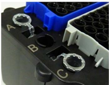
**Figure 3. Microcentrifuge tube slots.** Microcentrifuge tube slot B is not used in this protocol.
