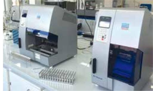
The EZ1 Advanced instrument which automates the critical RNA extraction step of the COVID-19 test.
