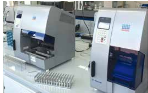
The EZ1 Advanced instrument which automates the critical RNA extraction step of the COVID-19 test.
