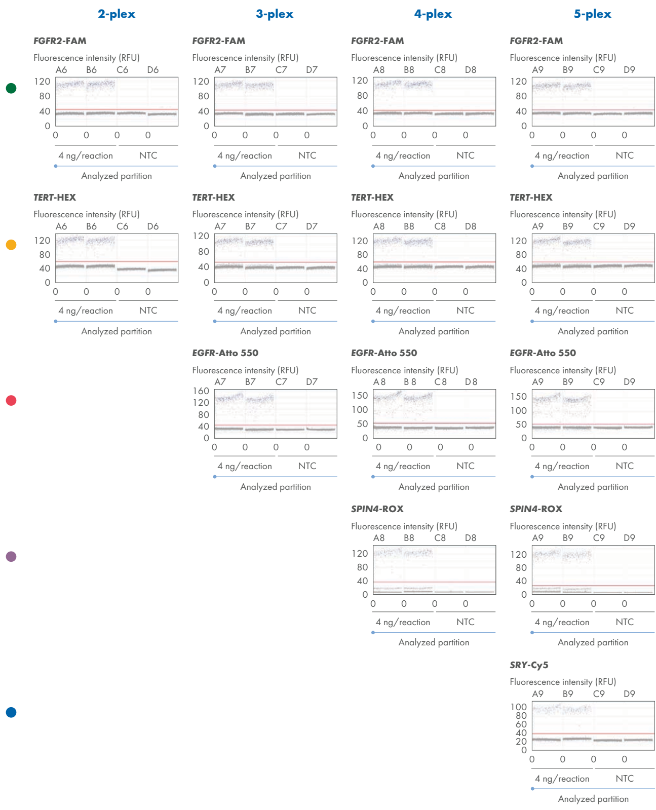
Five dPCR Probe CNV Assays were multiplexed in a single reaction using 4 ng of gDNA per reaction.
