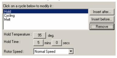
Select "Cycling" and set up the parameters for PCR cycling as shown below.
