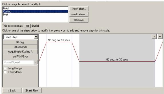
4. Select "Melt" and set up the parameters for melting curve analysis as shown below.
