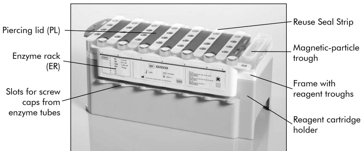
**Figure 5. QIA Symphony reagent cartridge (RC).** The reagent cartridge (RC) contains all reagents required for the purification procedure.
