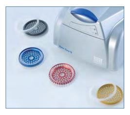
Multiple PCR tube and Rotor-Disc formats.
