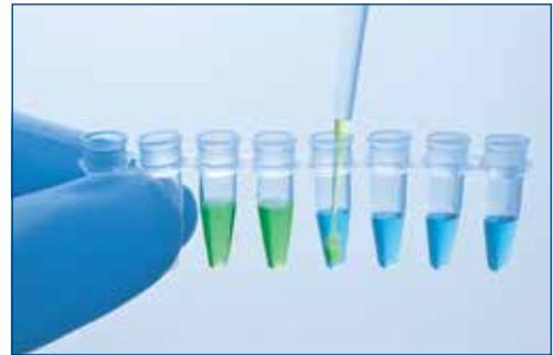
**Figure 2. Accurate reaction setup indicated by the built-in pipetting control.** The QuantiNova SYBR Green PCR Master Mix contains an inert blue dye. Combined with QuantiNova Yellow Template Dilution Buffer, the resulting solution turns green, indicating that the reaction was set up correctly.
