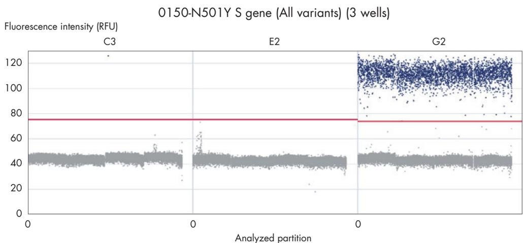
**Figure 6.** Fluorescence intensities as measured by the QIAcuity instrument in the CRIMSON (Cy5) channel. C3 = NTC; E2 = Negative donor; G2 = Positive donor for the UK variant.
