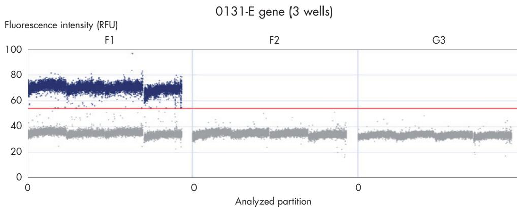
Figure 1. Fluorescence intensities as measured by the QIAcuity instrument. 0131-E gene: F1 = Positive donor; F2 = Negative donor; G3 = NTC.
