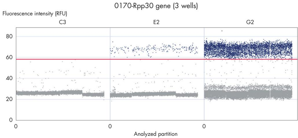
**Figure 7.** Fluorescence intensities as measured by the QIAcuity instrument in the ORANGE (TAMRA) channel. C3 = NTC; E2 = Negative donor; G2 = Positive donor for the UK variant.
