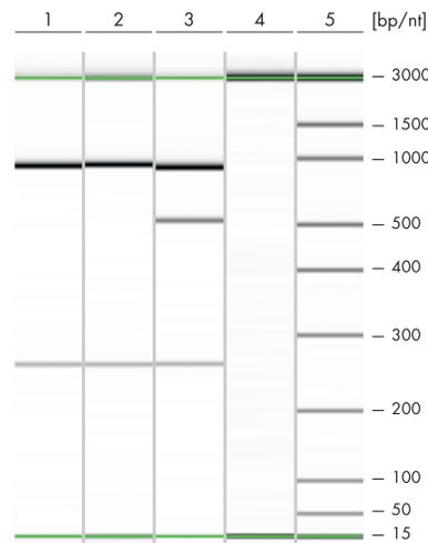
Gel image demonstrating detection of 16S rDNA, *nuc* and *mecA* genes using QIAXcel Advanced. Lanes 1, 2: *S. aureus* (*nuc*+); Lane 3: MRSA (*nuc*+, *mecA*+); Lane 4: NTC; Lane 5: DNA size marker.
