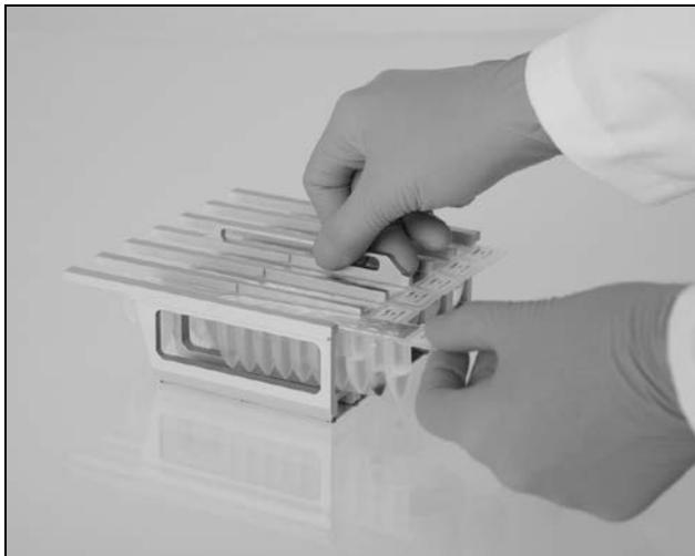
**Figure 3. Ease of instrument setup using reagent cartridges (RCV).** **A** A sealed, prefilled reagent cartridge (RCV). Fill levels vary, depending on the type of reagent cartridge (RCV). **B** Loading reagent cartridges (RCV) into the cartridge rack. The cartridge rack itself is labeled with an arrow to indicate the direction in which reagent cartridges (RCV) must be loaded.
