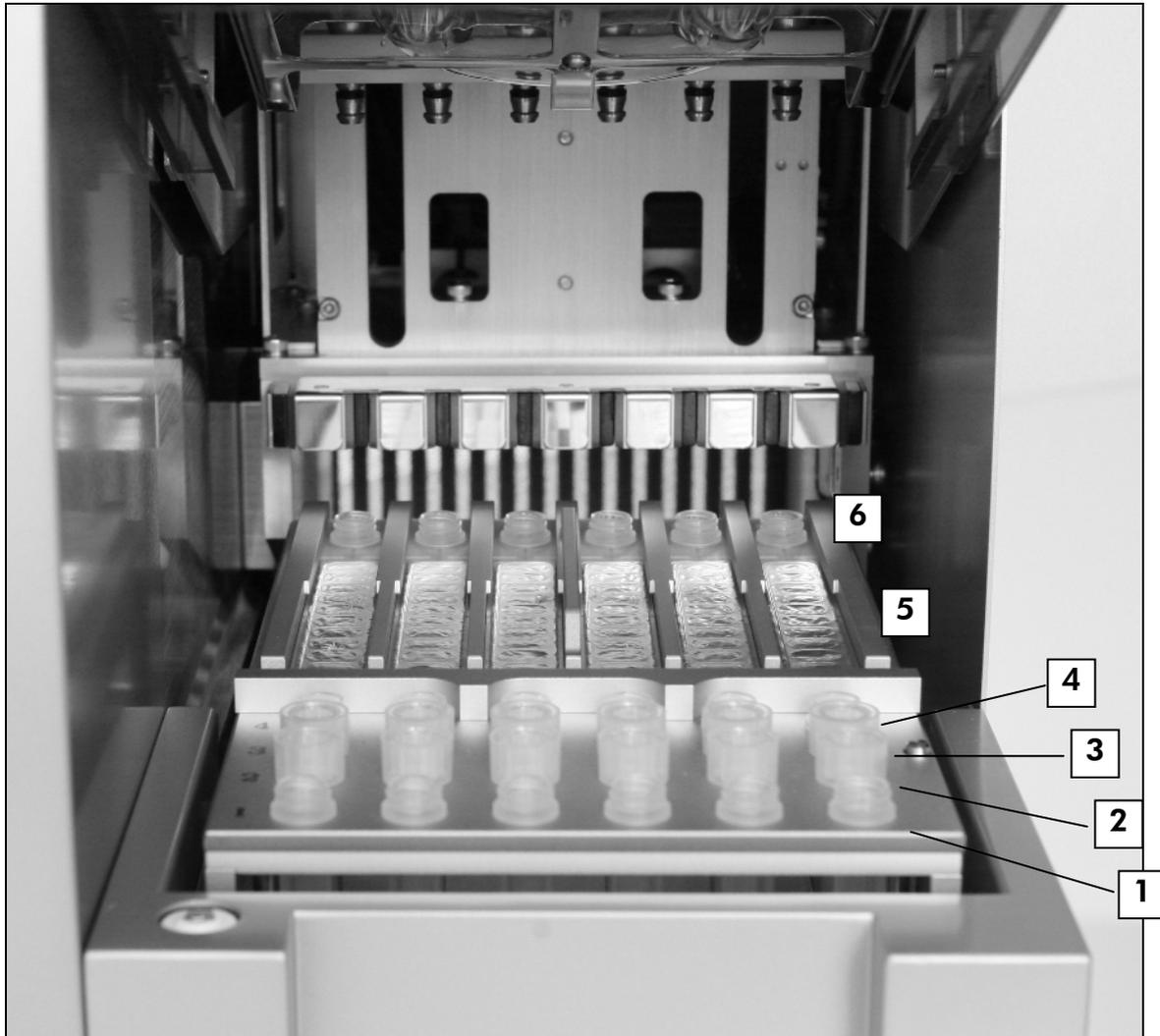
**Figure 4. Worktable of an EZ1 instrument.**
