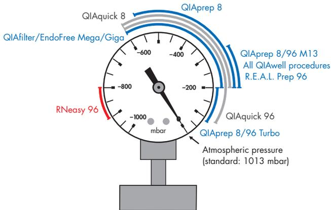
**Figure 6.** Schematic representation of recommended vacuum pressures for QIAGEN procedures.
