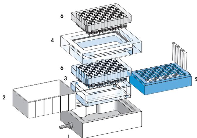
**Figure 4.** Components of the QIAvac 96 manifold.
