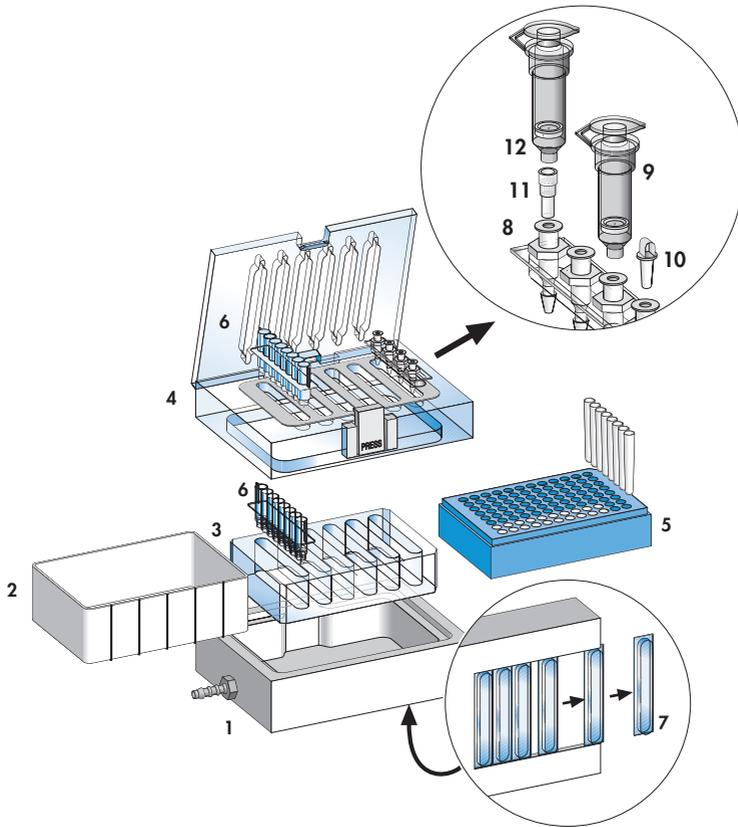
**Figure 3.** Components of the QIAvac 6S manifold.
