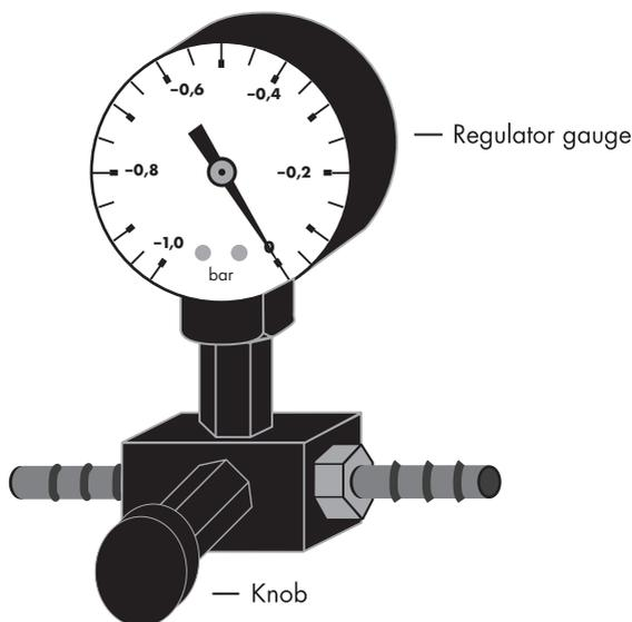
**Figure 5.** Schematic diagram of the Vacuum Regulator.
