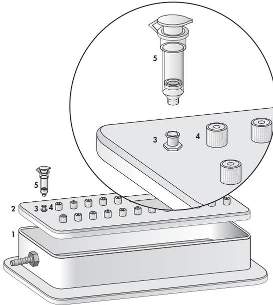
**Figure 1:** Setting up QIAvac 24 with QIAprep, QIAquick, MinElute, or RNeasy Mini spin columns.
