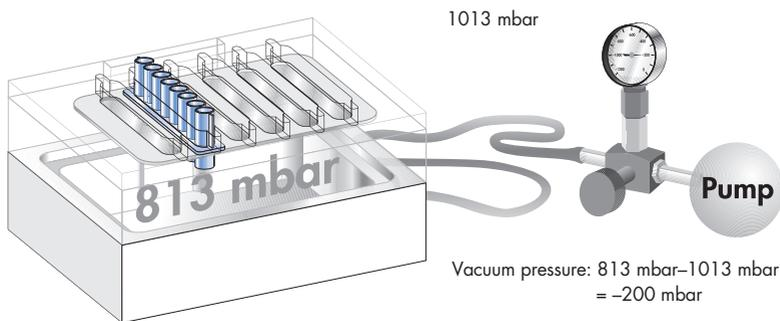
**Figure 7.** Definition of vacuum pressure
