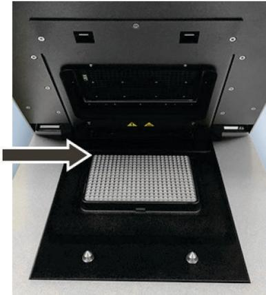
**Figure 7. Position A1 on the sample block.**
