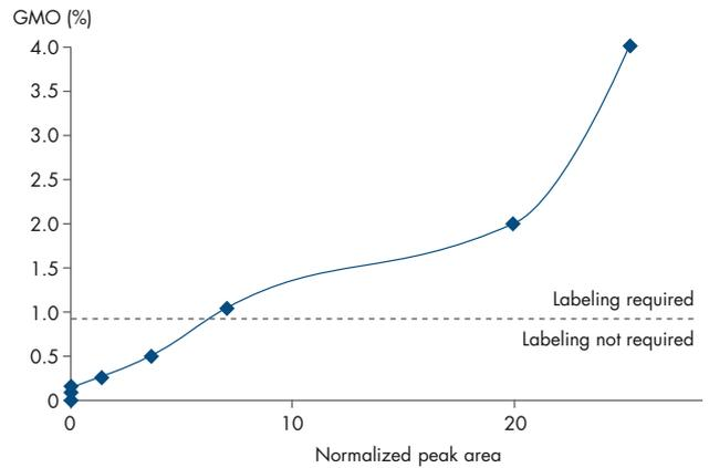
**Figure 2. LOD of the QIAxcel System.** The LOD was calculated for the quantitative normalized area (peak area) of the amplified 35S product at a defined number of copies per reaction. According to the EU GMO regulation, the limit of detection for a GMO marker must be below 0.9%. Food containing over 0.9% GMO content must be labeled.
