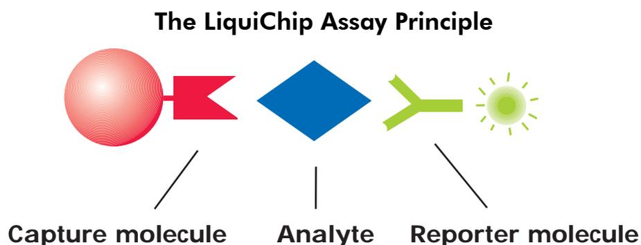
**Figure 1** The LiquiChip assay principle. Analytes free in solution interact with bead-bound capture molecules and are detected using reporter molecules specific for the analyte.
