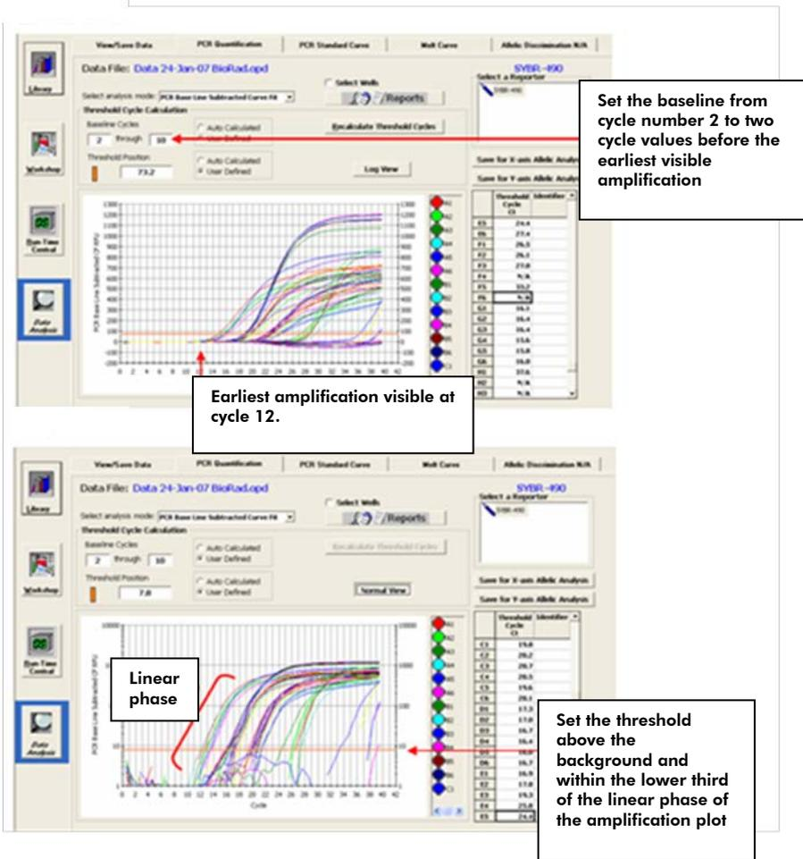
Figure 5. Setting the baseline and threshold values.
