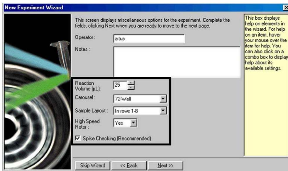
Fig. 3: Setting of General Assay Parameters.
