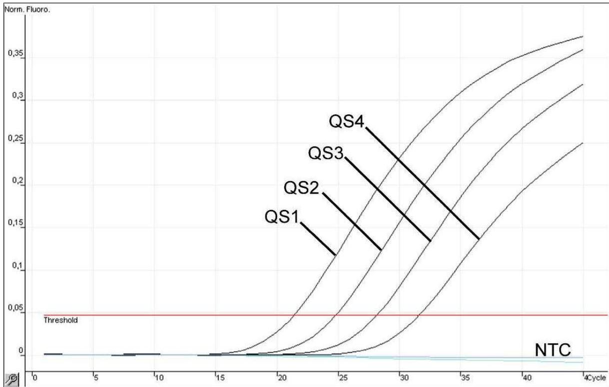
Fig. 9: Detection of the *Quantitation Standards* (SARS-CoV LC/RG/TM QS 1 – 4) in fluorescence channel Cycling A.FAM. NTC: non-template control (negative control).
