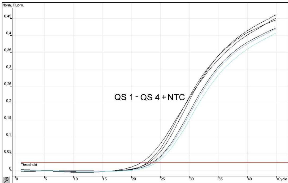
Fig. 10: Detection of the *Internal Control* (IC) in fluorescence channel Cycling A.JOE with simultaneous amplification of the *Quantitation Standards* (SARS-CoV LC/RG/TM QS 1 – 4). NTC: non-template control (negative control).
