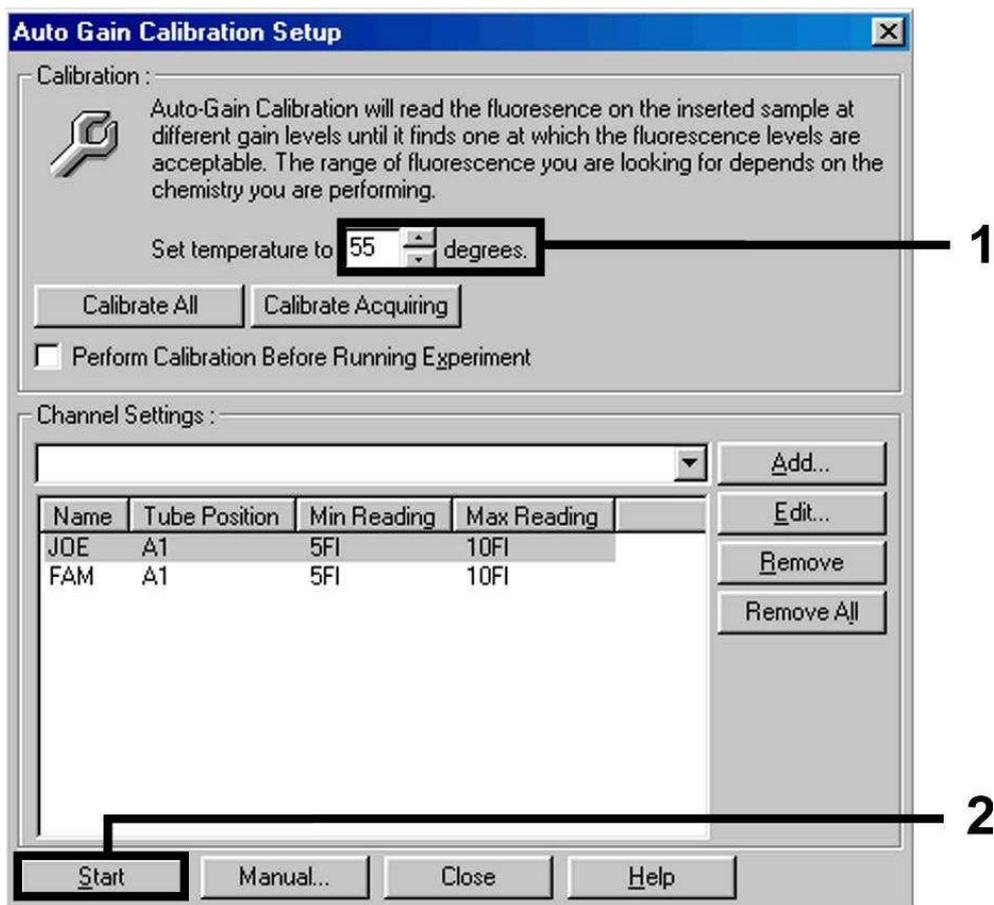
Fig. 7: Adjustment of the Fluorescence Channel Sensitivity.
